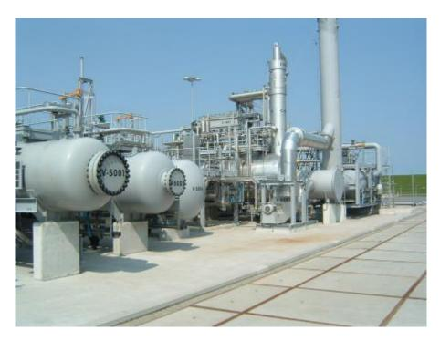
To convert a gas or steam into liquid; to improve distillation efficiency by means of condensation in a reflux process.
